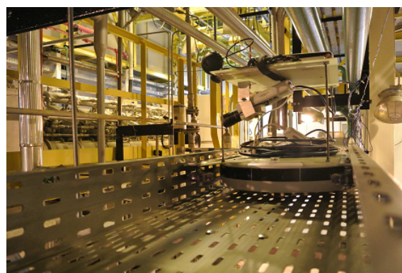
Figure 5.3: General setup of database recording using a moving camera on a robotic platform.
