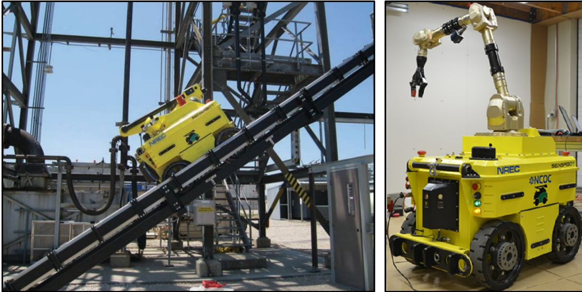
Figure 1.4: Sensabot being tested in an offshore environment. (NREC/CMU 2012)
