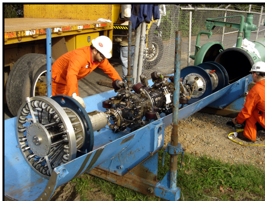
(a) A Pipeline Inspection Gauge (PIG).
