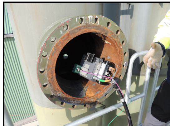
(b) PETROBOT's vessel inspection robot.
