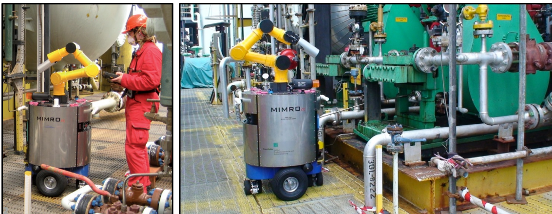
Figure 1.3: MIMROex being tested on an offshore facility. (Bengel & Pfeiffer 2007)
