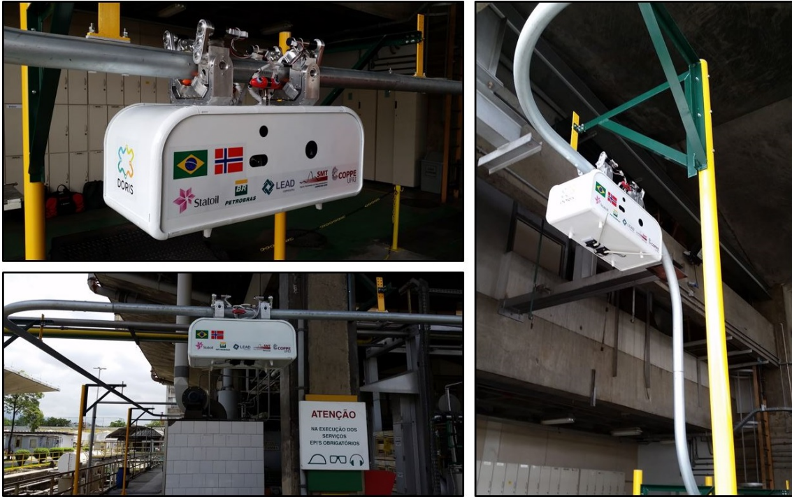
Figure 3.1: Pictures of DORIS operating in a test at an utility plant at Petrobras-CENPES.
