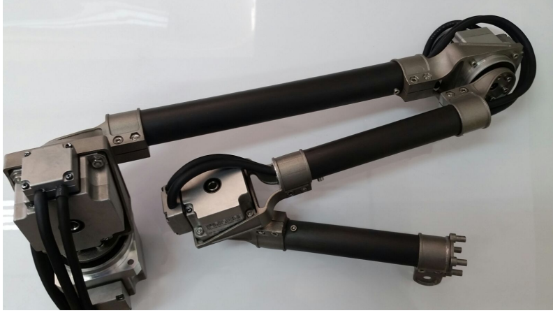
Figure 5.1: Manipulator TETIS under construction at a bench test.
