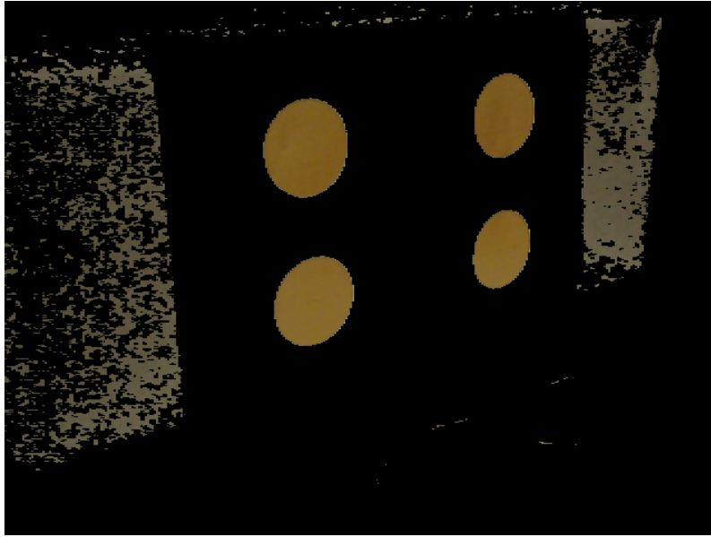
Figure 4.9: Result of bitwise operation with HSV mask, applied to the original image.
