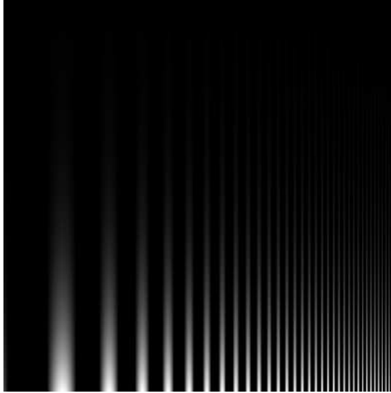
Figure 2.8: Chart illustrating the dependence between contrast perception and spatial frequencies of the image. The frequency of the pattern increases horizontally, from left to right. All illuminated patches, between the dark patches, have their intensities vertically decreasing at the same rate, from the highest intensity (bottom row) to the lowest intensity (top row). The perceived height of the illuminated patches changes according to the spatial frequency (expressed in cycles/degree).
