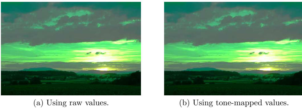
Figure 3.28: Application of the White Patch algorithm to the digital FPTMO output image, before demosaicing: (a) white-balance gain computation based on maximum raw pixel values at each color channel; (b) white-balance gain computation based on maximum tone-mapped pixel values at each color channel.
