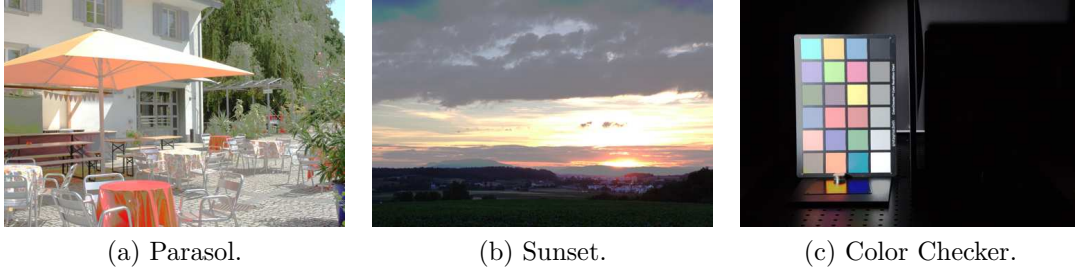
Figure 3.18: Results from the FPTMO first digital version, which uses the average raw pixel value of the input image to perform the tone mapping on all pixels, regardless of the color channel that each pixel represents.
