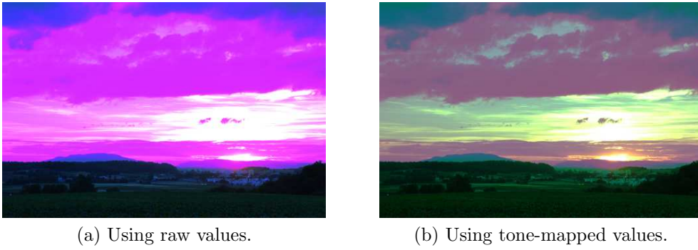
Figure 3.26: Images obtained after applying the Gray World white-balance algorithm to the tone-mapped image before the demosaicing. In (a) and (b), the average values of each color channel are calculated using the raw pixel values and the tone-mapped pixel values, respectively.
