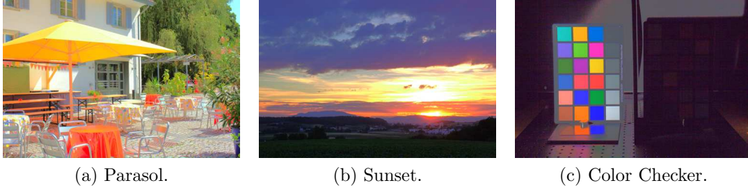
Figure 3.38: Color images resulting from the fourth FPTMO digital implementation, in which the red and blue pixel integration times are determined by the neighboring green pixel.
