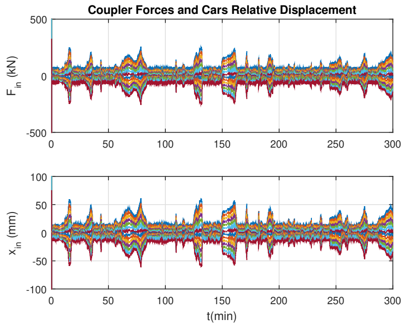
Figure 4.28 – Simulation results of a 15 cars train with the real terrain and a time varying speed reference. The couplers force time history. The speed reference is tracked. Distributed power and air braking are exploited.
