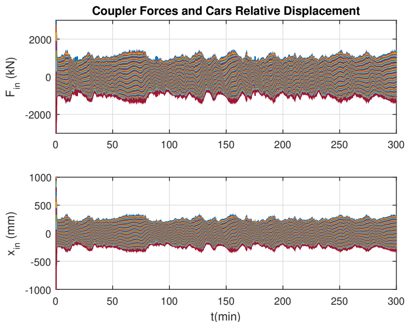
Figure 4.33 – Simulation results of the 71 cars train with the MPC approach and a time varying speed reference. The coupler forces time history. Distributed power and air braking are exploited.
