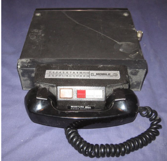
(a) A radio telephone from 0G [2].
