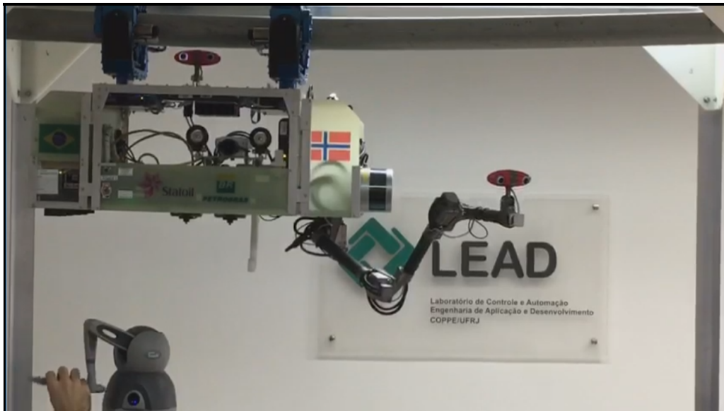
Figure 1.5: Doris Project, a mobile robot for offshore inspection developed by GSCAR, Petrobras and Statoil.
