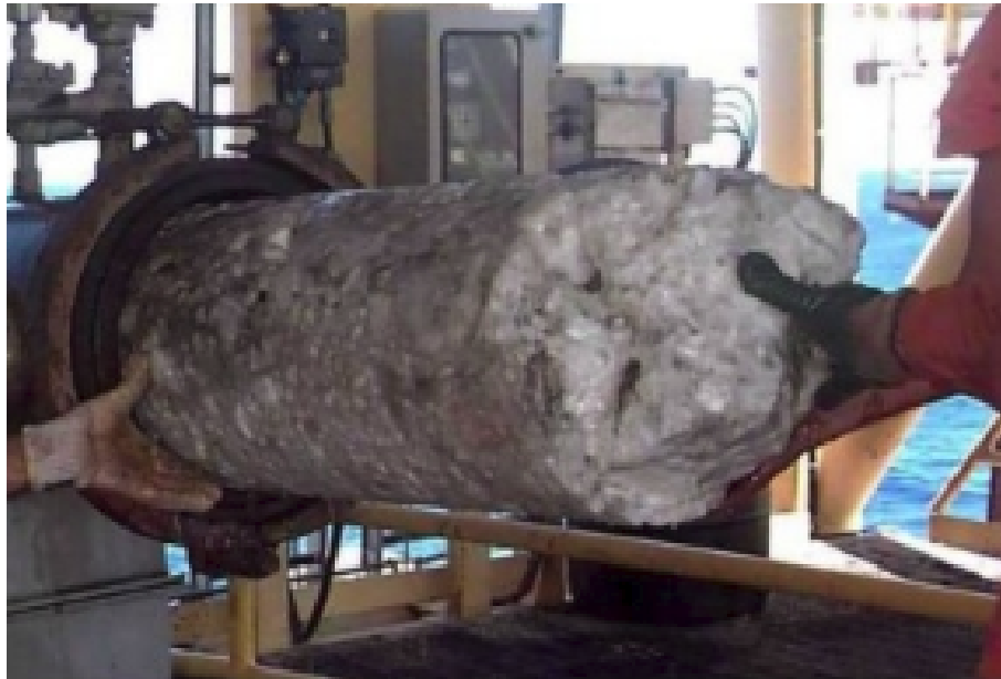
Figure 2.2: Illustration of the removal of a hydrate plug from a pipeline showing that the process is not simple and that the hydrate plug can completely jam the pipeline. Source [1].
