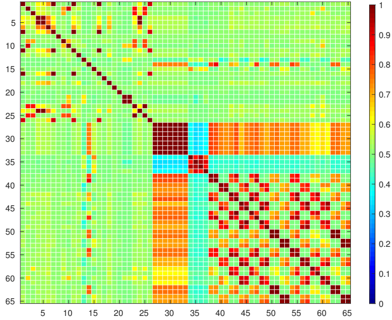
Figure 3.7: Correlation matrix of all features used in the ISCX botnet dataset. Features from 1 to 26 are the initial features inferred from the packet headers of IP-IP flow, and features 37 to 65 are obtained through the graph-based enrichment.
