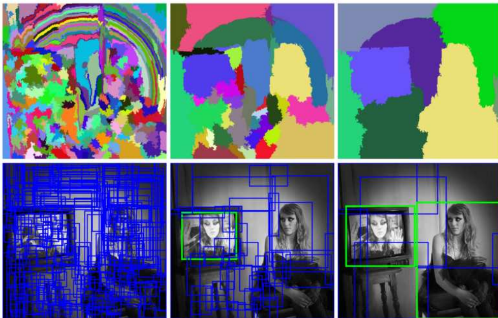
Figure 4.2: Selective search example. The first row are the combined regions, the blue and green boxes in the second row are the possible RoI and detected objects, respectively. Source: [87].
