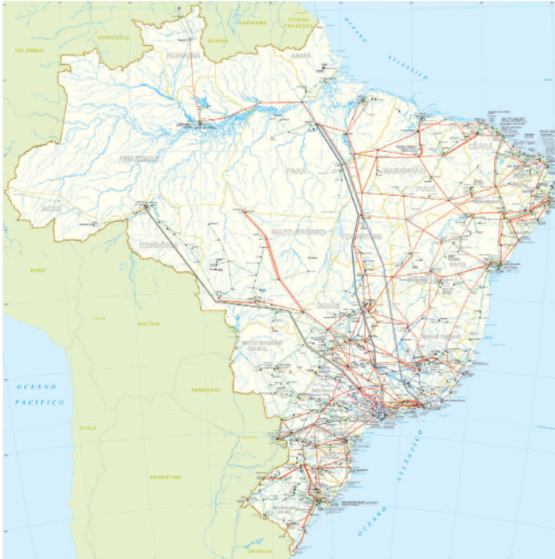
Figure 4.40: Brazilian Interconnected Power System (BIPS).
