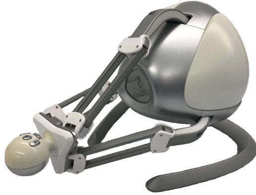
Figure 3.16: 3-DoF teleoperation device used in experiments.
