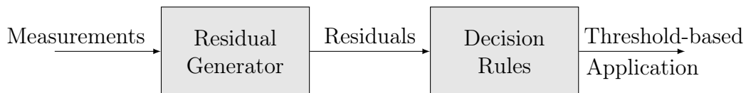
Figure 2.4: General Framework for Fault Detection.
