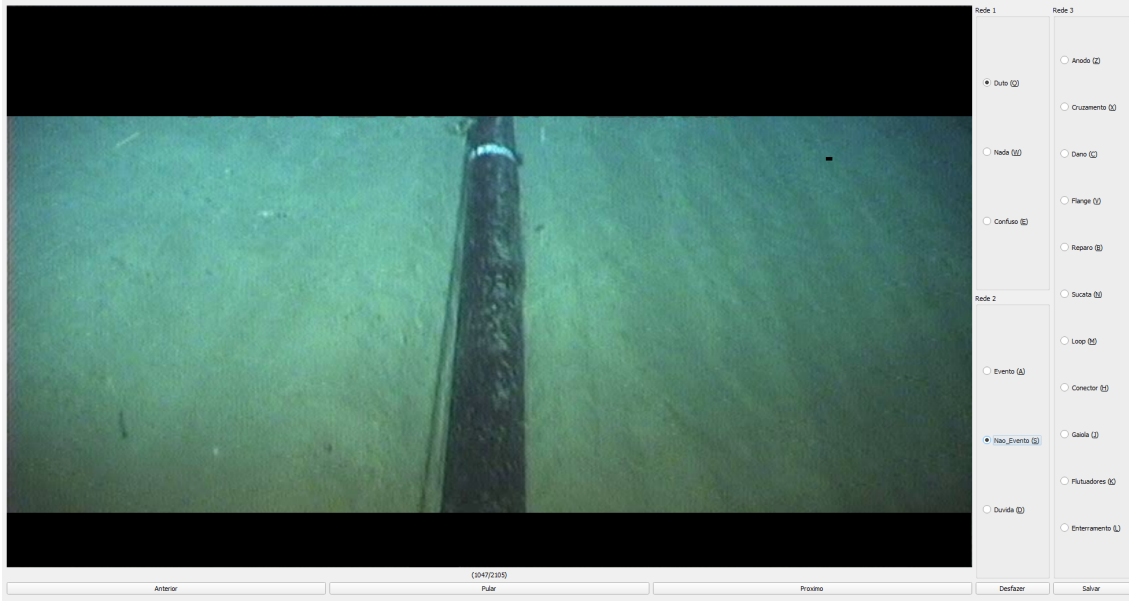
Figure 2.2: Screen capture of the labeling interface in use. The top and bottom portions of the image are omitted. The rightmost portion of the screen displays buttons used to assign labels for the three classification levels described in Section 3.2. The user selected the classes Duct, for level 1, and Not Event, for level 2.
