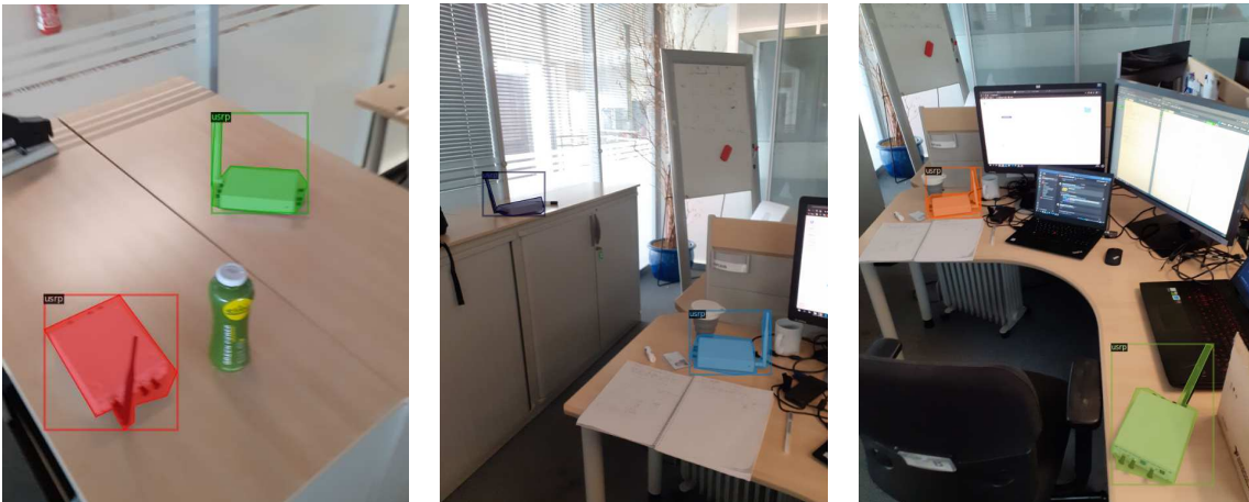
Figure 2.3: Examples of manually annotated images with bounding boxes around USRPs, used for fine-tuning the model pre-trained on the COCO dataset.
