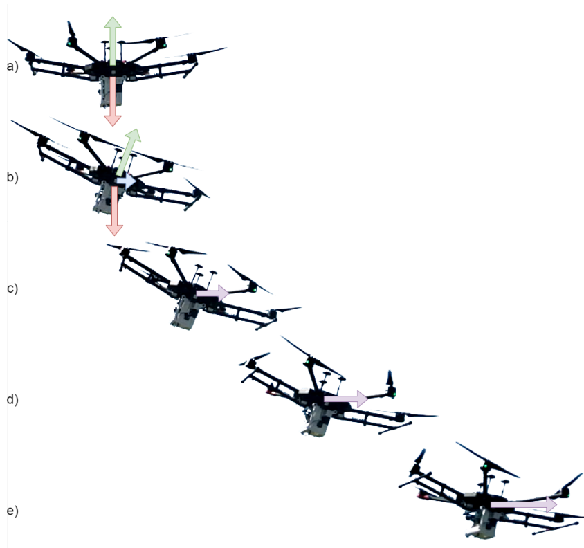
Figure 2.7: DJI M600 Pro Accelerating in level flight. In (a) and (b): Red arrow represents gravity, green arrow represents net aerodynamic acceleration, blue arrow represents net acceleration. In (c)–(e): Purple arrows represent velocity vectors at each instant.
