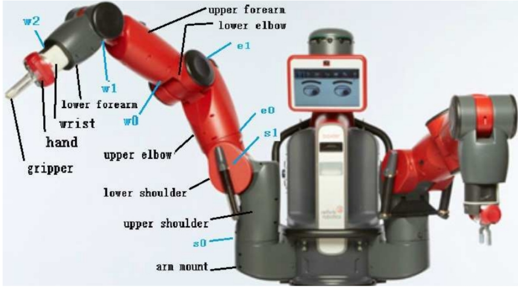
Figure 4.2: The arms of Baxter robot, from [38].
