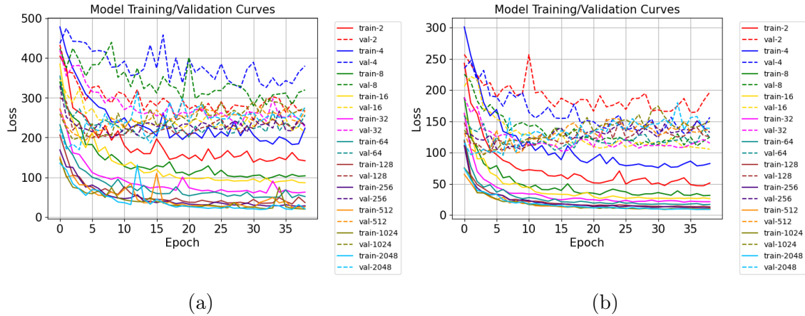
Figure 5.7: Training and validation curves for the models in (a) private-PBTDB and (b) crowd-PBTDB. Solid lines indicate training performance, whereas dashed lines indicate validation performance.
