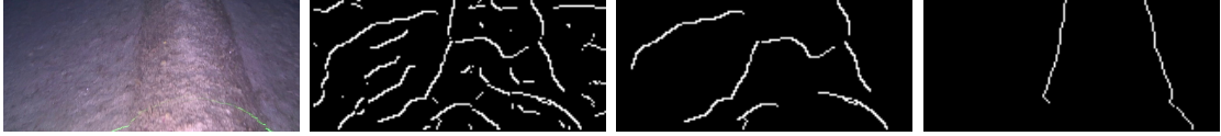
Figure 2.8: Color edge detection. From left to right: input image, color edge detector [1], color edge detector [1] combined with edge score, proposed color edge detector with \theta = \frac{\pi}{2} . All pixel values > 0 were set to 1 for visualization.
