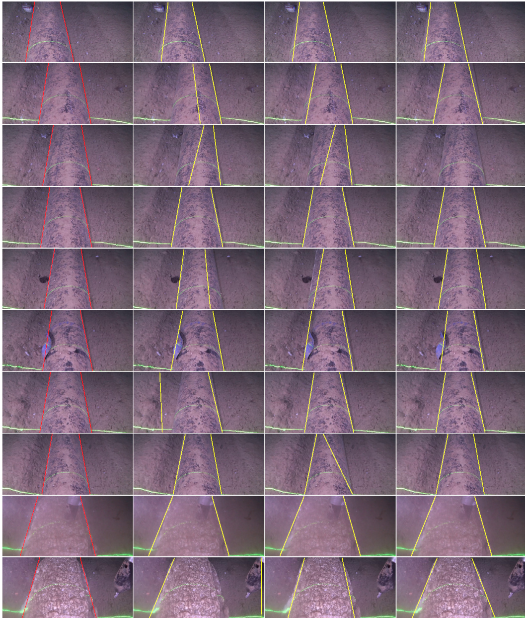
Figure 3.7: Detection example from video 5. From left to right: ground truth (red), tracking using 2, 5 and 9 frames (yellow).
