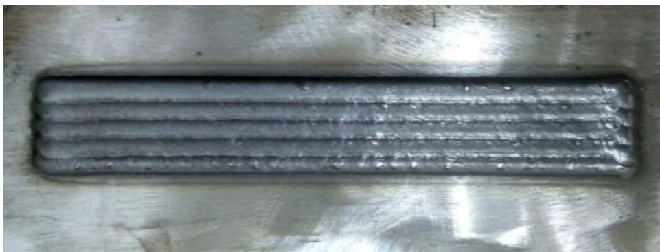
Figure 6.8: Five bead layer sample of the second experiment. The deposition of all bead are performed in the same direction.
