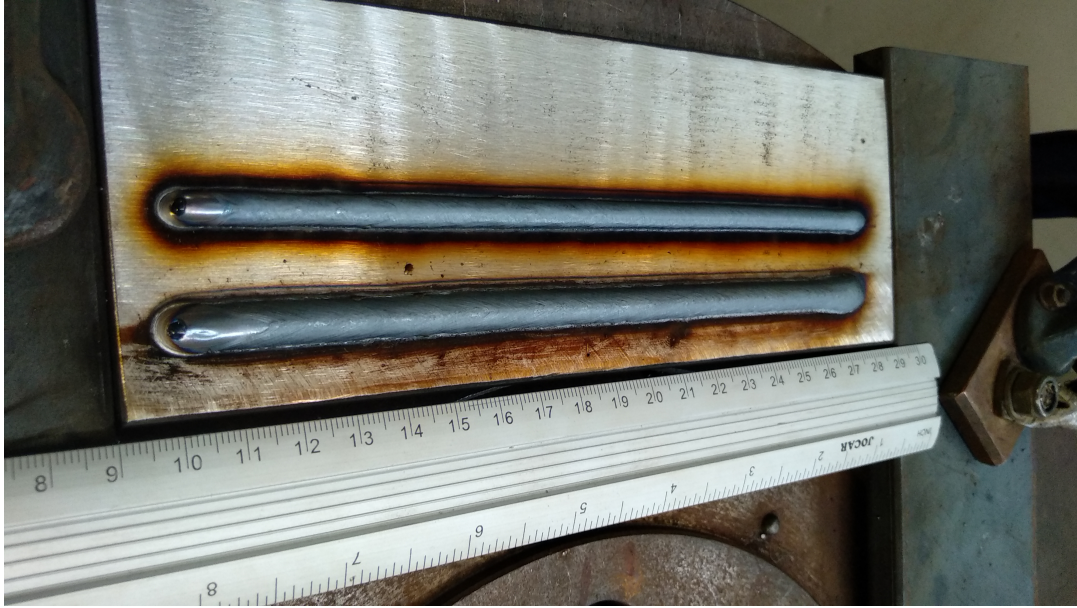
Figure 6.3: Single-bead specimens of the first experiment.
