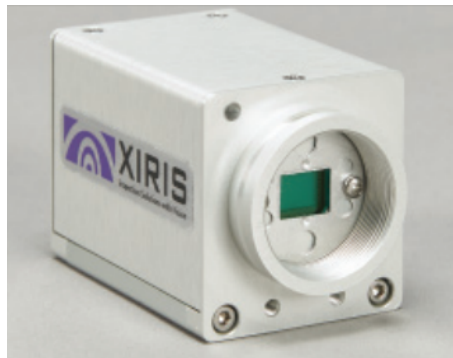
Figure 6.2: Gray-scale camera from Xiris used during metal deposition.
