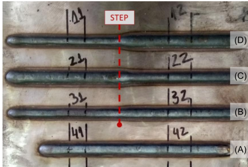
Figure 6.7: Samples of the second single-bead experiment with constant and varying wire feed speed (Table 6.3).
