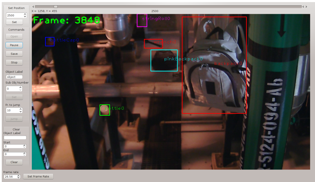
Figure 4.11: Example of abandoned-object annotation with the help of the developed annotation tool.
